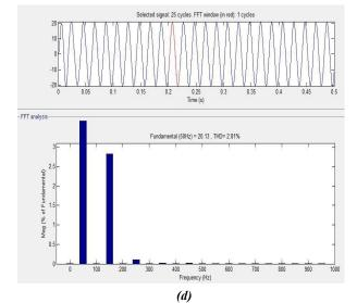
Fig.8. (a) Five level Output voltage of inverter and grid voltage(b) In phase waveform of grid voltage and grid current (c) Active and Reactive power of inverter (d) Harmonic Analysis of Grid Current
