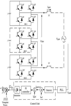
Fig.4. Circuit diagram of Cascaded Seven level Inverter for single phaseGrid Connected System
