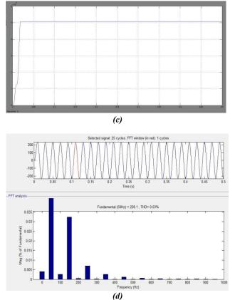
Fig.12.(a) Nine level Output voltage of inverter and grid voltage (b) Inphase waveform of grid voltage and grid current (c) Active and Reactive Power of inverter (d) Harmonic Analysis of Grid Current.
