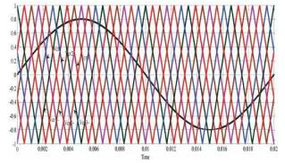
Fig.3. Phase shift PWM for seven-level inverter
